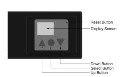
**RESET on End Plate switch:** Should you encounter any problems where the door may require a reset, you need to press and hold the select button and then press & release the hidden Reset button that is located in the <u>Top right Hand</u> corner of the Grey membrane.
