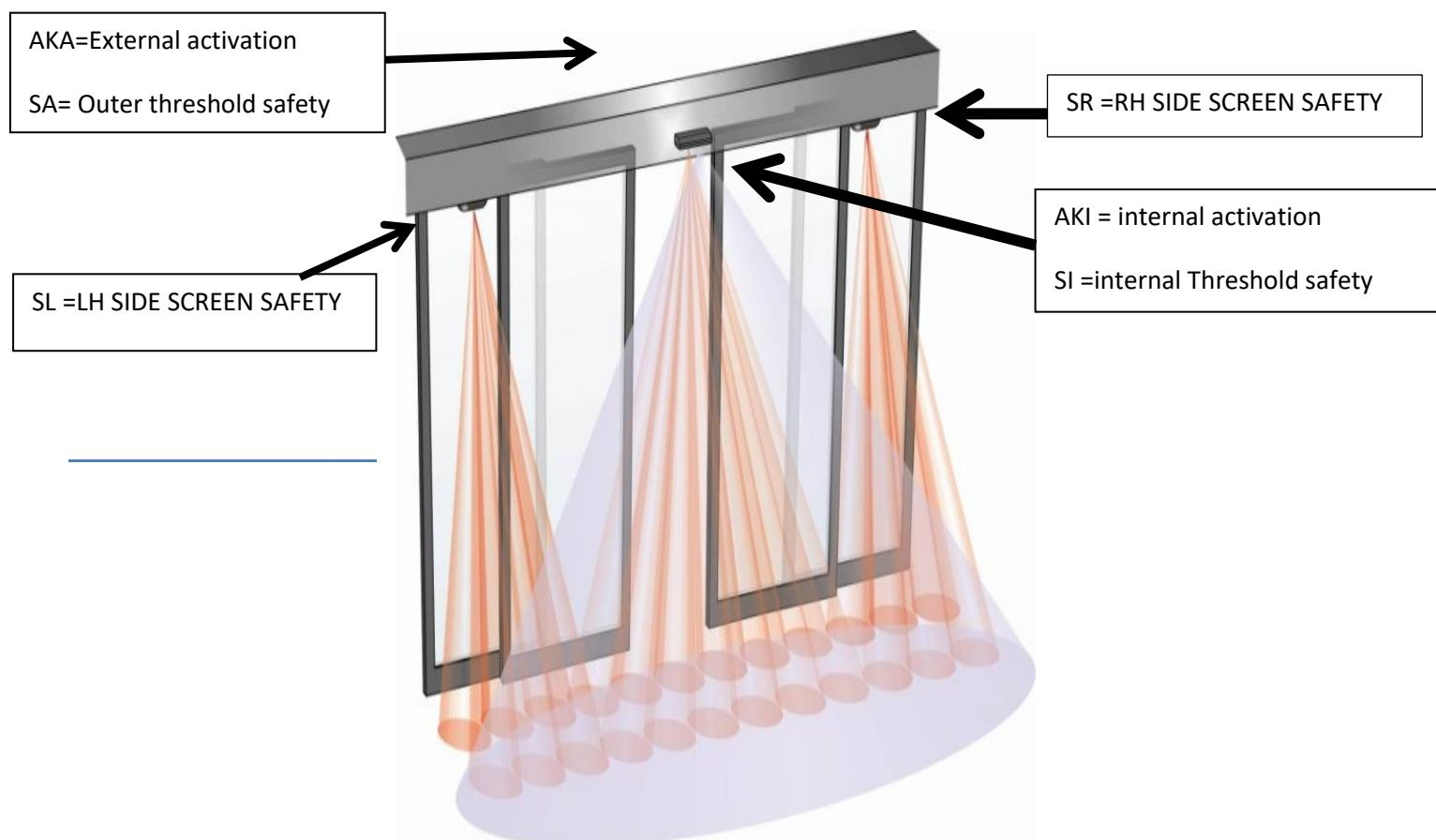
There are several adjustable parameters for each sensor. Please treat the Activation and safety of each sensor as separate entities.
