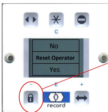
For final exit of the building, place the program selector into the locked function and when you are ready to leave press the lock symbol once to give a single open/close exit.
